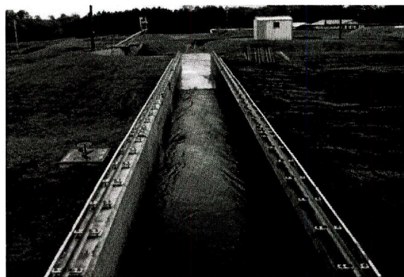
Figure 8. Open channel erosion test on bare earth channel.
