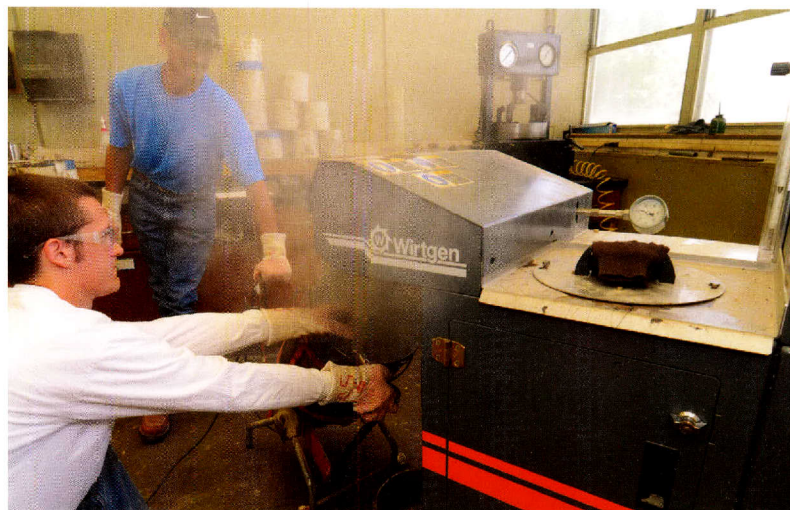
Staff members confirm proper foaming of the asphalt in TTI’s laboratory foaming plant prior to mixing test batches for the mixture design.
