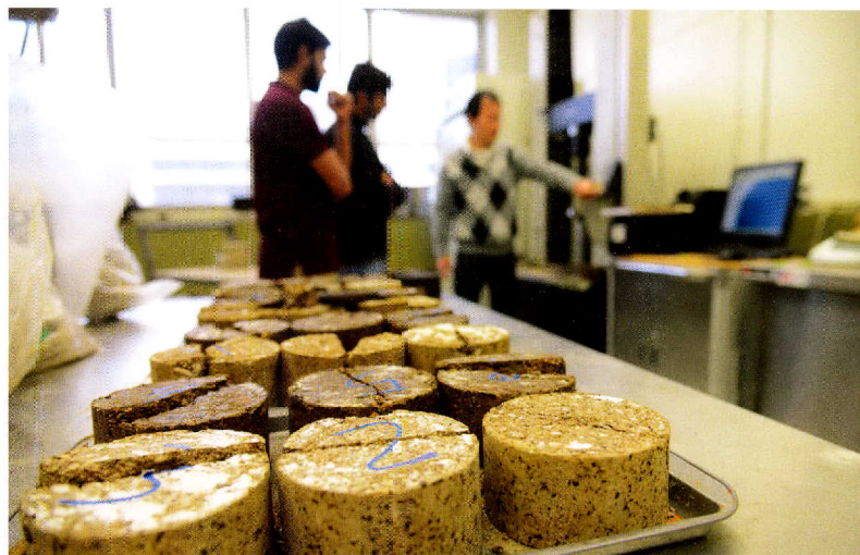
These samples of recycled pavement were treated with foamed asphalt to develop full-depth recycling options for using existing pavement in rehabilitating roadways — a more cost-effective and environmentally friendly approach compared to rebuilding the entire roadway from scratch.
