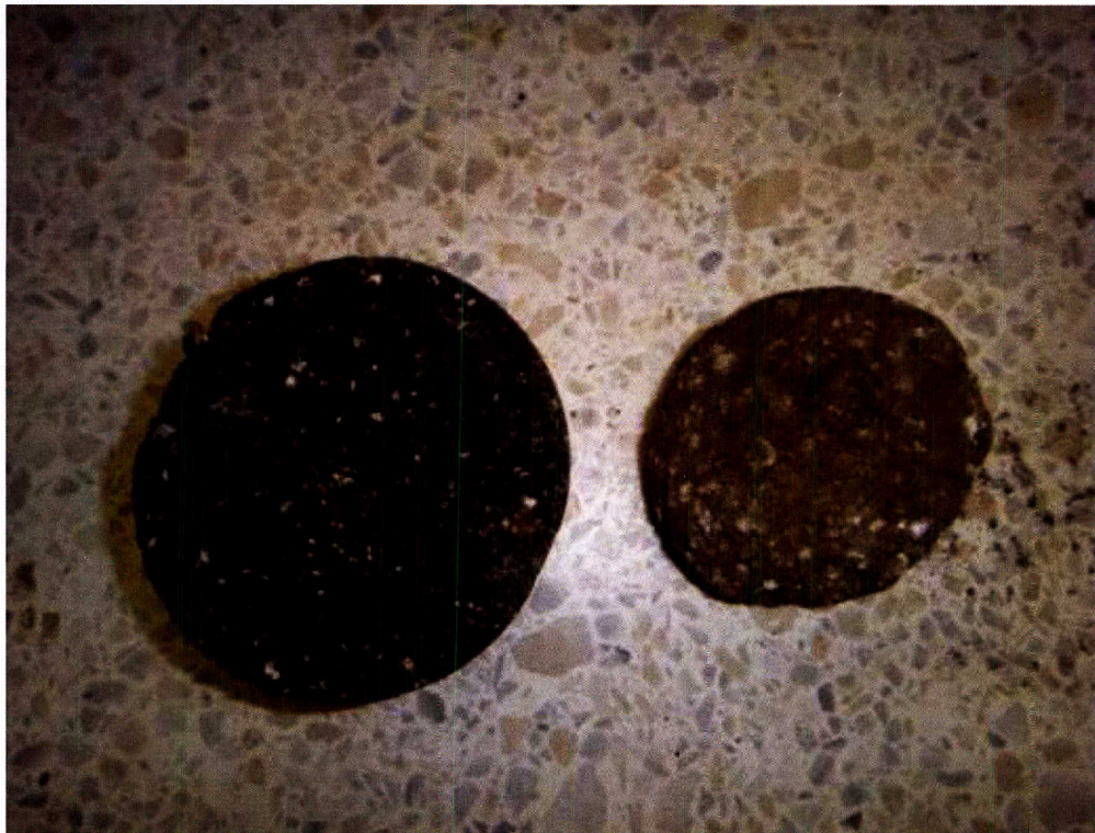
Figure 16. Texas Gyratory LRA Specimen before and after Cantabro Test.
