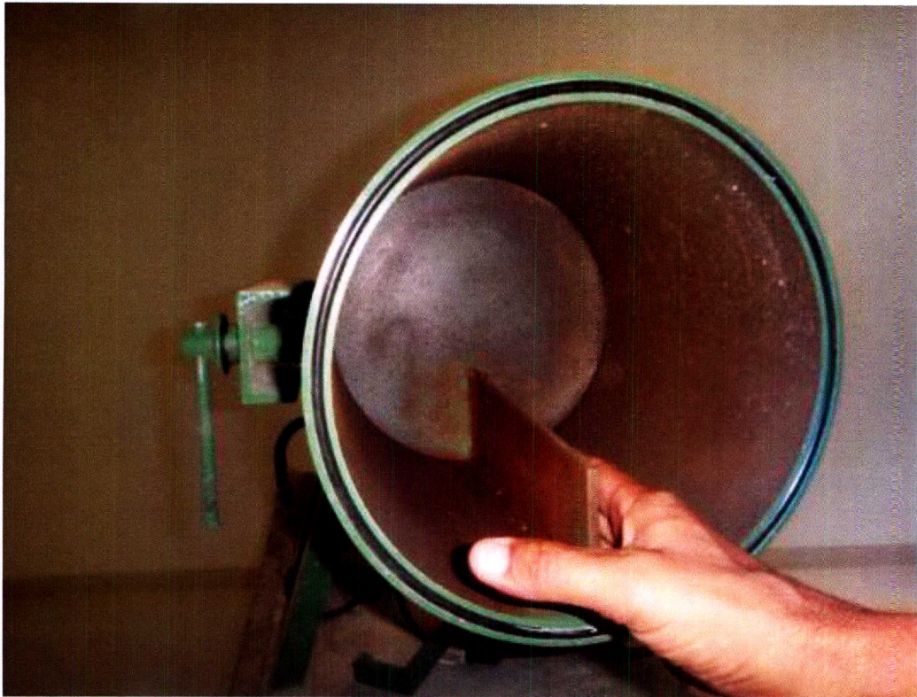
Figure 11. Inside of Wet Ball Mill Drum.
