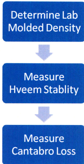
Figure 23. Proposed Testing Sequence for Single Texas Gyratory Molded Specimen.
