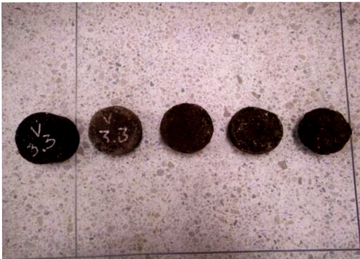
Figure 17. Cantabro-Tested Specimens at Decreasing Flux Oil Contents from Left to Right.
