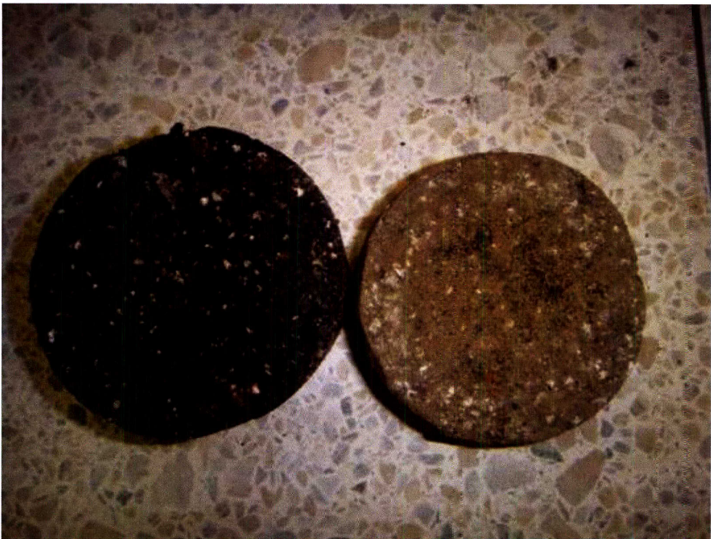
Figure 12. Texas Gyratory Specimen of LRA before and after Tumbling in Wet Ball Mill Machine.
