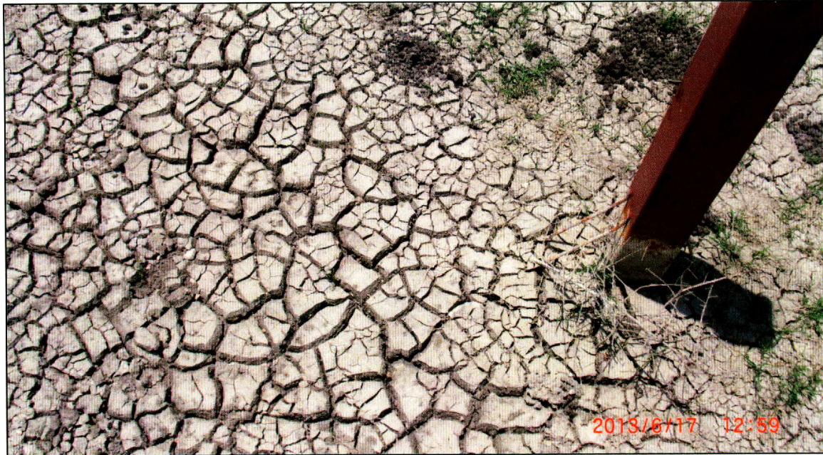
Figure 5.27: Inundation zone on June 17, 2013, 2 weeks into second drying cycle. Stand pipe piezometer casing is 4" across.
