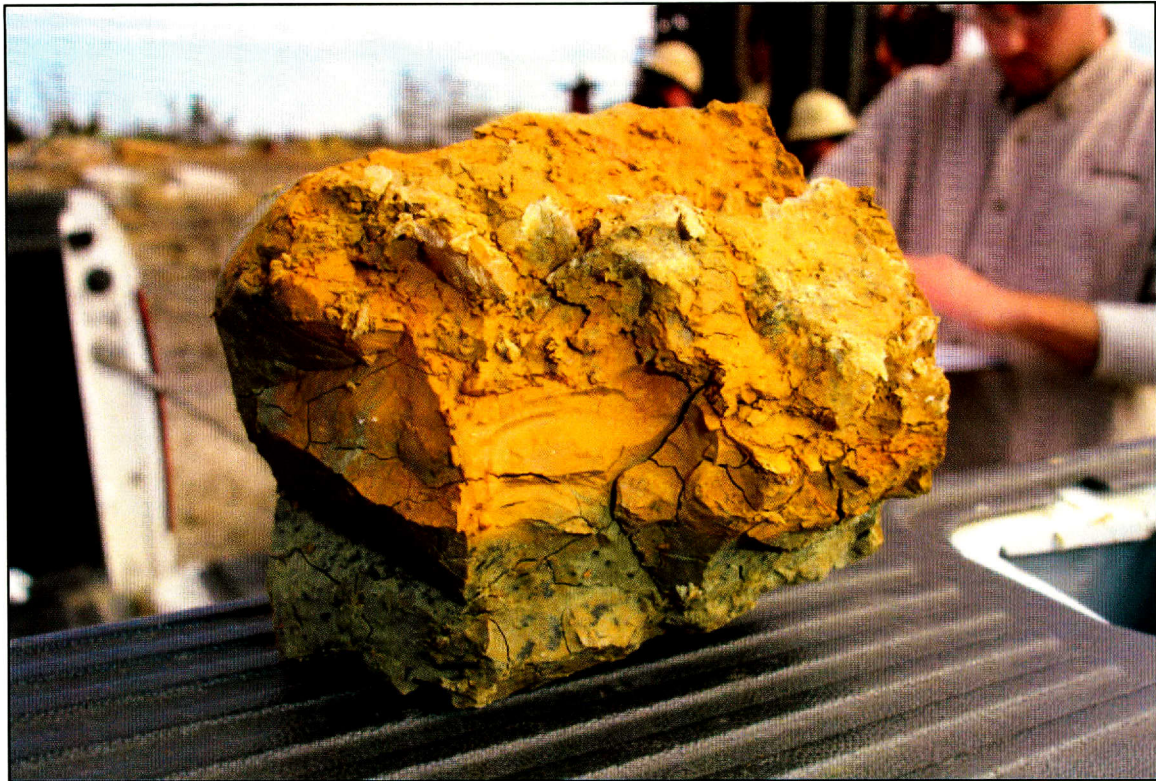
Figure 4.3: Unweathered Taylor Clay from the project site in Manor.
