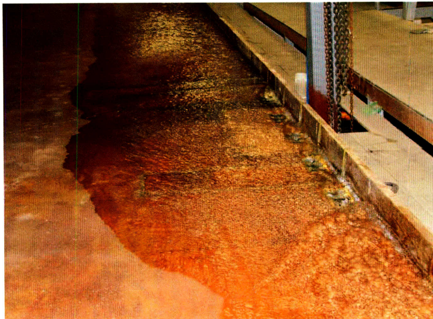
Figure B-6 Flow Profile (Looking Upstream) with 5-open 4in. × 8in. Drains at 4% Cross Slope and 1.0% Longitudinal Slope with Q = 2.25 Revolutions at Head Box Valve
