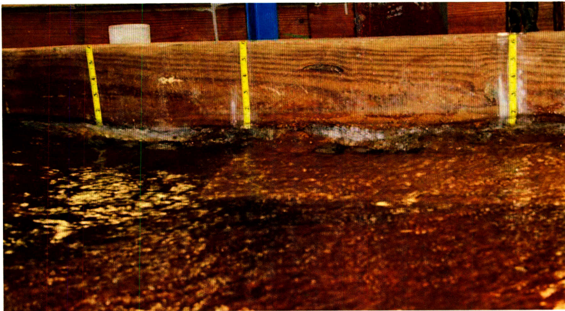
Figure B-10 Flow Depth against Curb Flow with 2-open 4in. × 8in. Drains at 4% Cross Slope and 0.1% Longitudinal Slope with Q = 1.5 Revolutions at Head Box Valve
