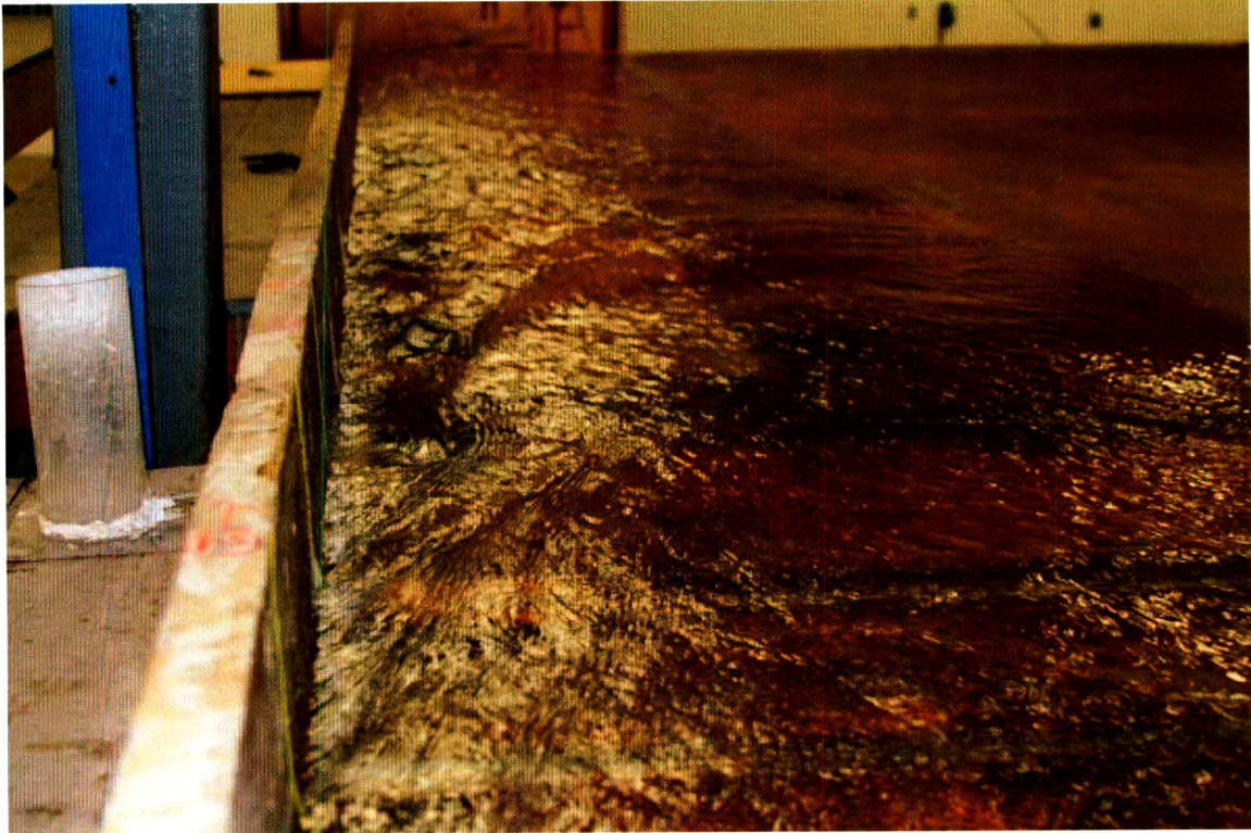
Figure B-9 Flow Pattern over Drains (Looking Downstream)
