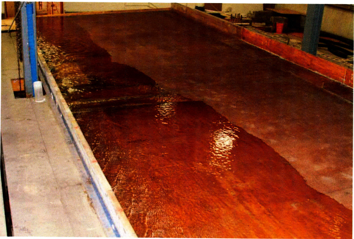
Figure B-8 Flow Profile (Looking Downstream) with 2-open 4in. × 8in. Drains at 4% Cross Slope and 0.1% Longitudinal Slope with Q = 1.5 Revolutions at Head Box Valve
