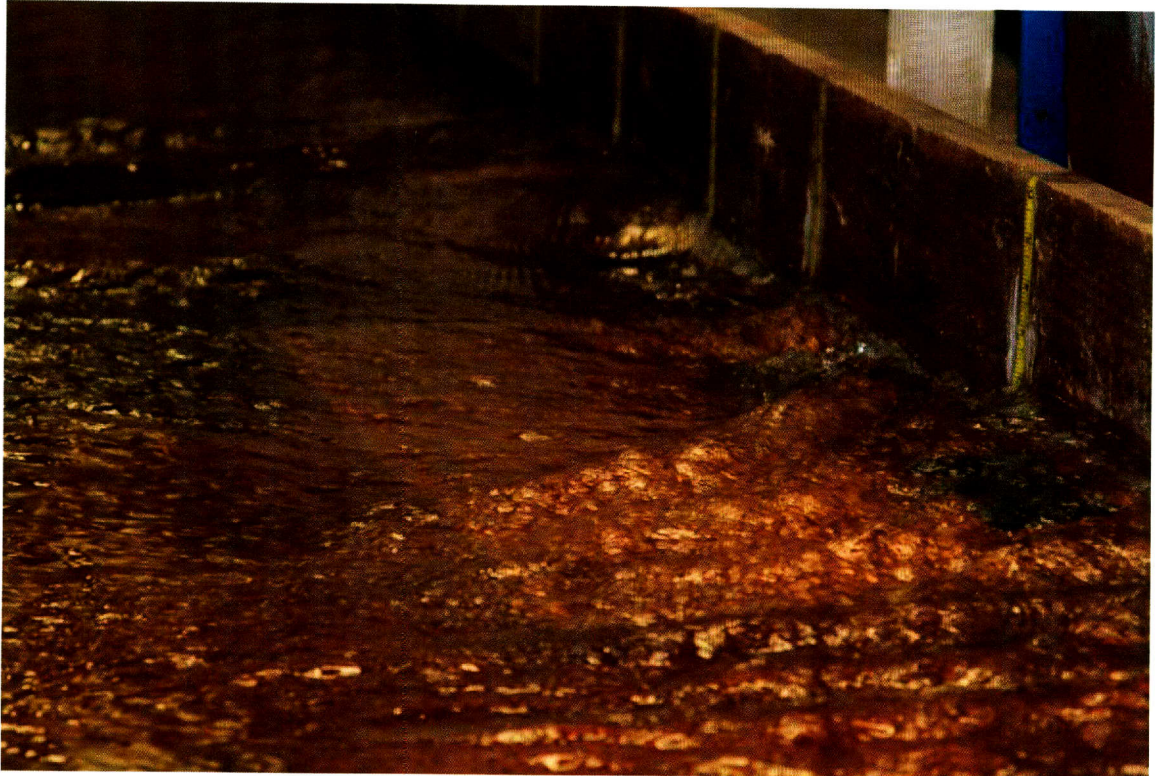
Figure B-11 Flow (Looking Upstream) with 2-open 4in. × 8in. Drains at 4% Cross Slope and 0.1% Longitudinal Slope with Q = 1.5 Revolutions at Head Box Valve
