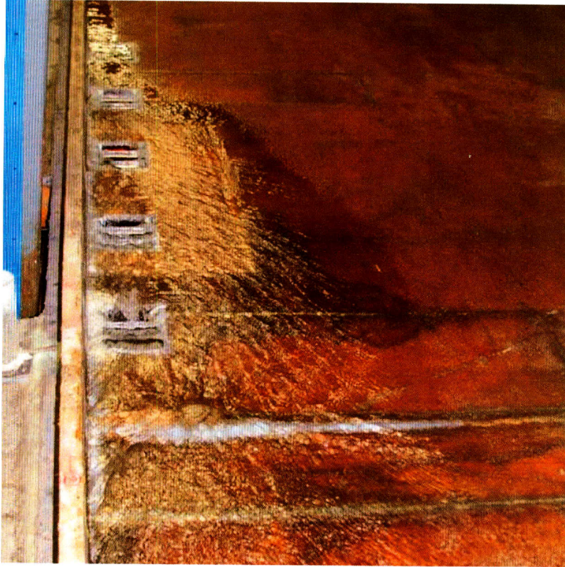
Figure B-19 Flow with 4-open 6in. × 8in. Drains at 6% Cross Slope and 0.5% Longitudinal Slope with Q = 1.25 Revolutions at Head Box Valve
