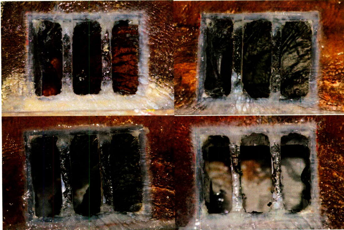
Figure B-17 Flow from the Right (upstream) into Drains 1 (top-left), 2 (top-right), 3 (bottom-left) and 4 (bottom-right) with 4-open 6in. × 8in. Drains at 2% Cross Slope and 0.5% Longitudinal Slope with Q = 1.0 Revolutions at Head Box Valve
