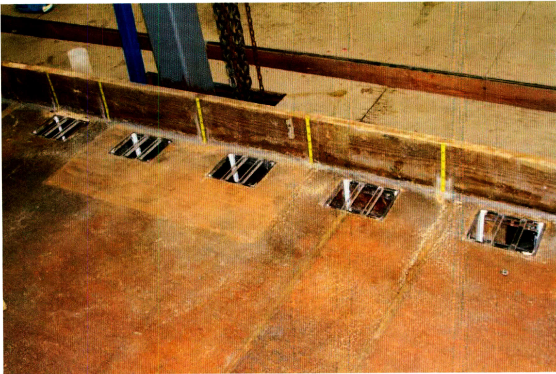
Figure 3-4 Plexiglas Drain Installments along Model Roadway
