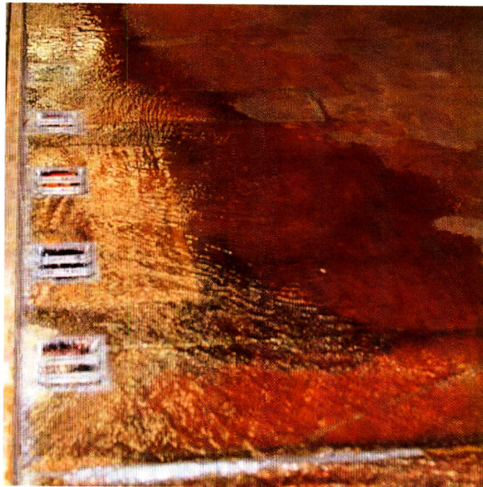
Figure B-16 Flow with 4-open 6in. × 8in. Drains at 2% Cross Slope and 0.5% Longitudinal Slope with Q = 1.0 Revolutions at Head Box Valve
