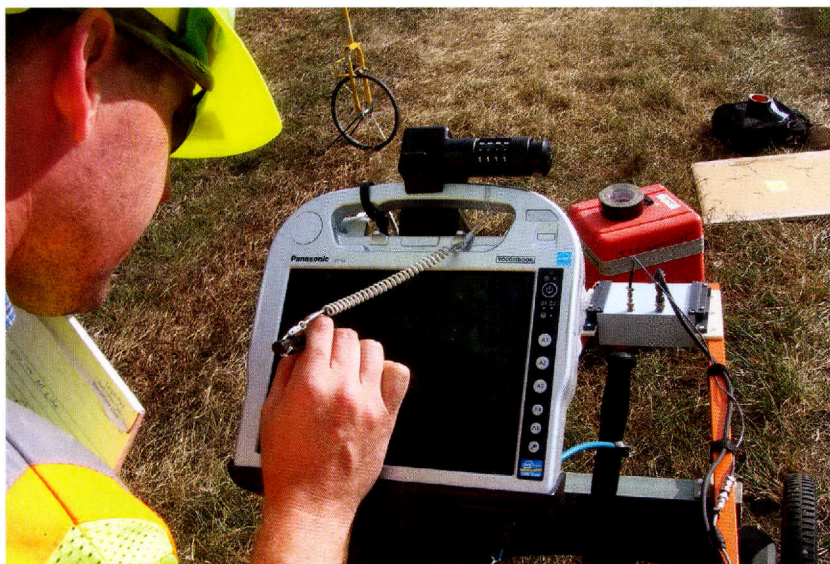
A technician evaluates the mix-density data collected from the new TTI-developed rolling density meter.
