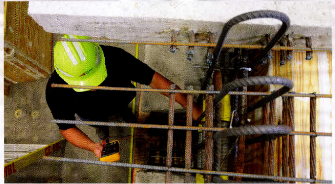
Researcher testing strain-gauge connections in one of the three spliced sections of the 71-foot concrete girder.
