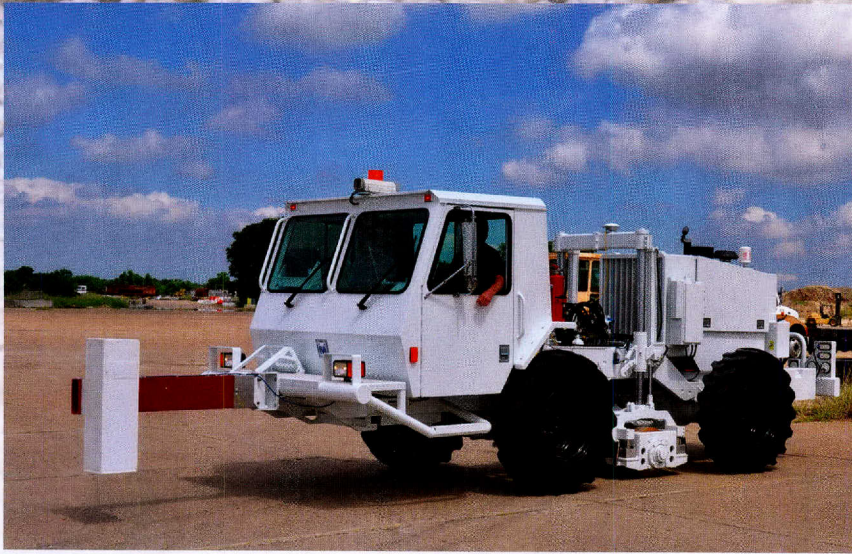
The total pavement acceptance device is now being used to identify defects within concrete pavements.
