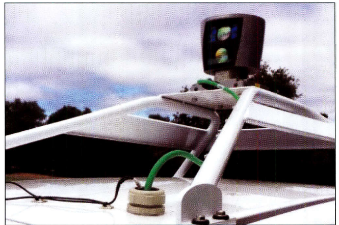
Lidar and GPS hardware on one of Google's self-driving cars.
