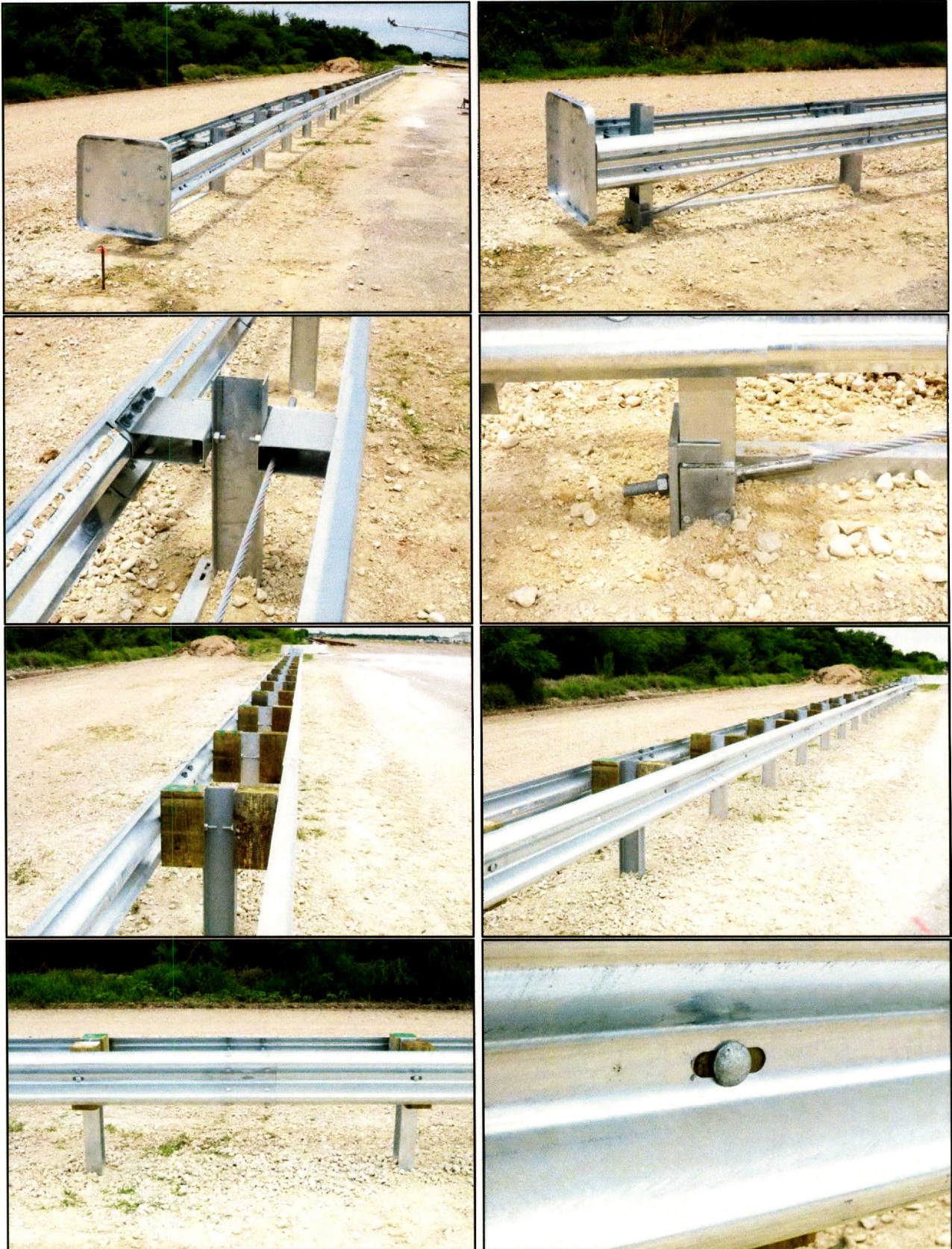
Figure 3.3. TxDOT 31-Inch W-Beam Median Barrier before Testing.
