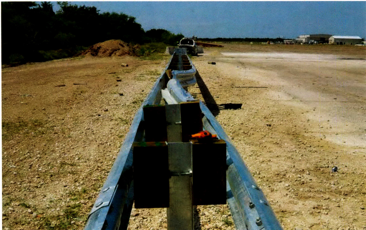
Figure 6.3. Vehicle/Installation Positions after Test No. 490023-3.
