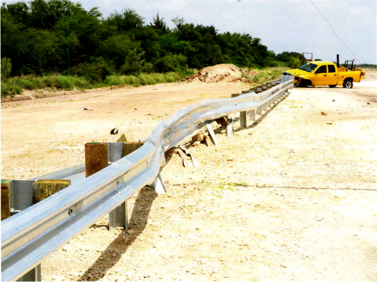
Figure 7.3. Vehicle/Installation Positions after Test No. 490023-4.
