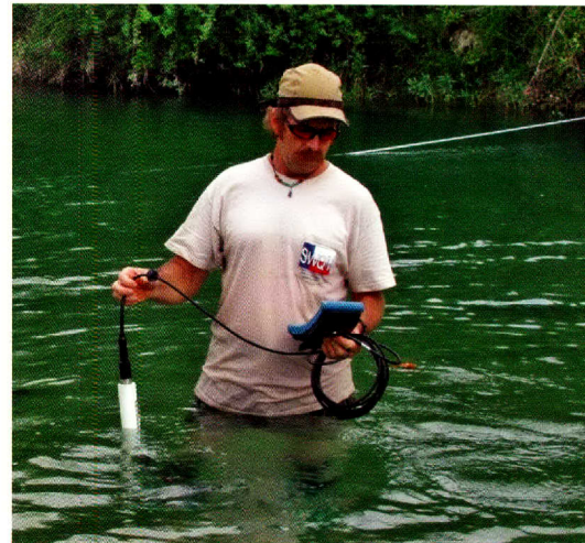
TCEQ SWQM staff member Bill Harrison uses the Hydrolab water quality monitoring device.
