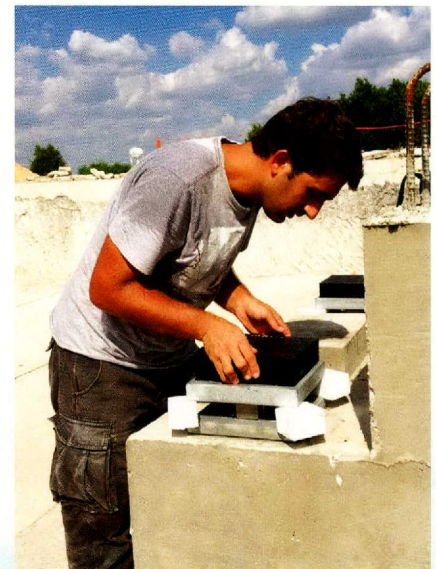
Tevfik Terzioglu, TTI graduate student, installs load cells and bearing pads for the bridge during testing.
