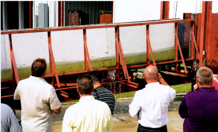
(Above and below) The variable slope channel flume is used for testing the performance capabilities of flexible channel liner materials at a range of stress flows.
