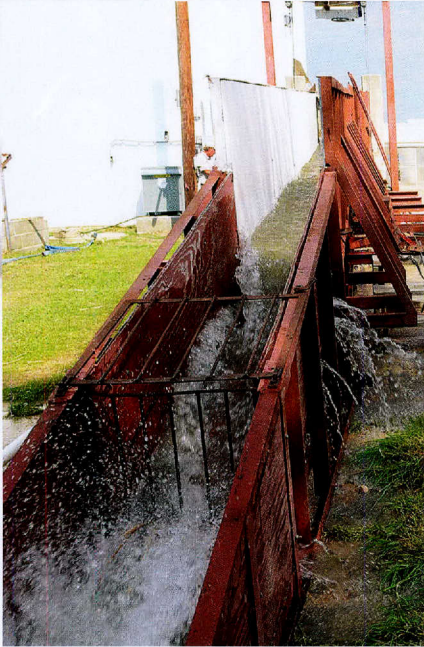
(Above and below) The variable slope channel flume is used for testing the performance capabilities of flexible channel liner materials at a range of stress flows.
