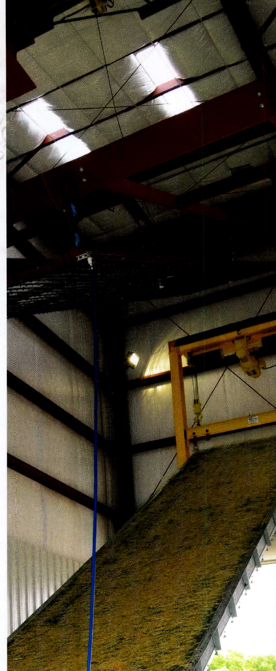
The rainfall simulators can adjust to match any desired slope up to 2:1 (50 percent) and accommodate any type of soil fill for research.
