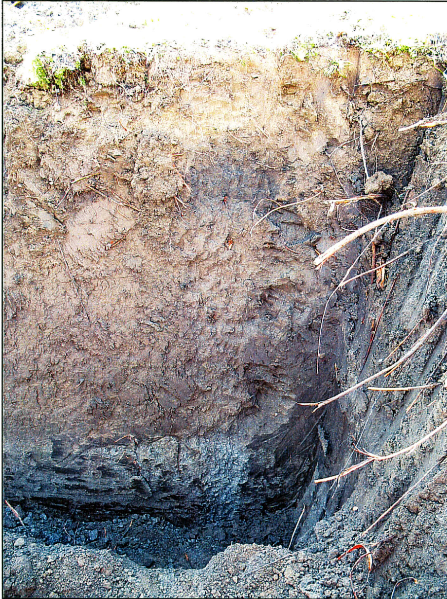
Figure 5. Backhoe trench 1. Note the amount of calcium carbonate in the bottom zone which ranges from 171 to 235 cm below the ground surface. View is to the south.
