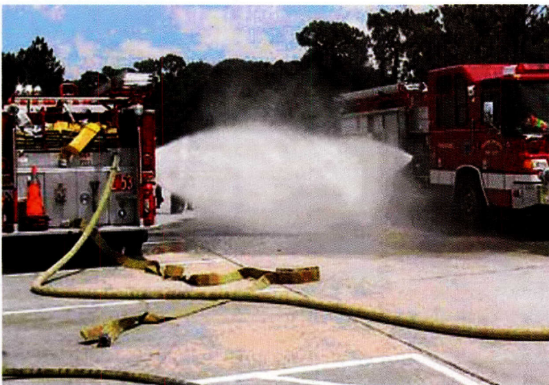
Figure 6—several methods exist to provide decontamination solution to a hasty decon. Soap and water or just plain water will work well under most conditions. Garden hoses, fire pumper trucks, fire hydrants, even buckets and sponges can be used.
