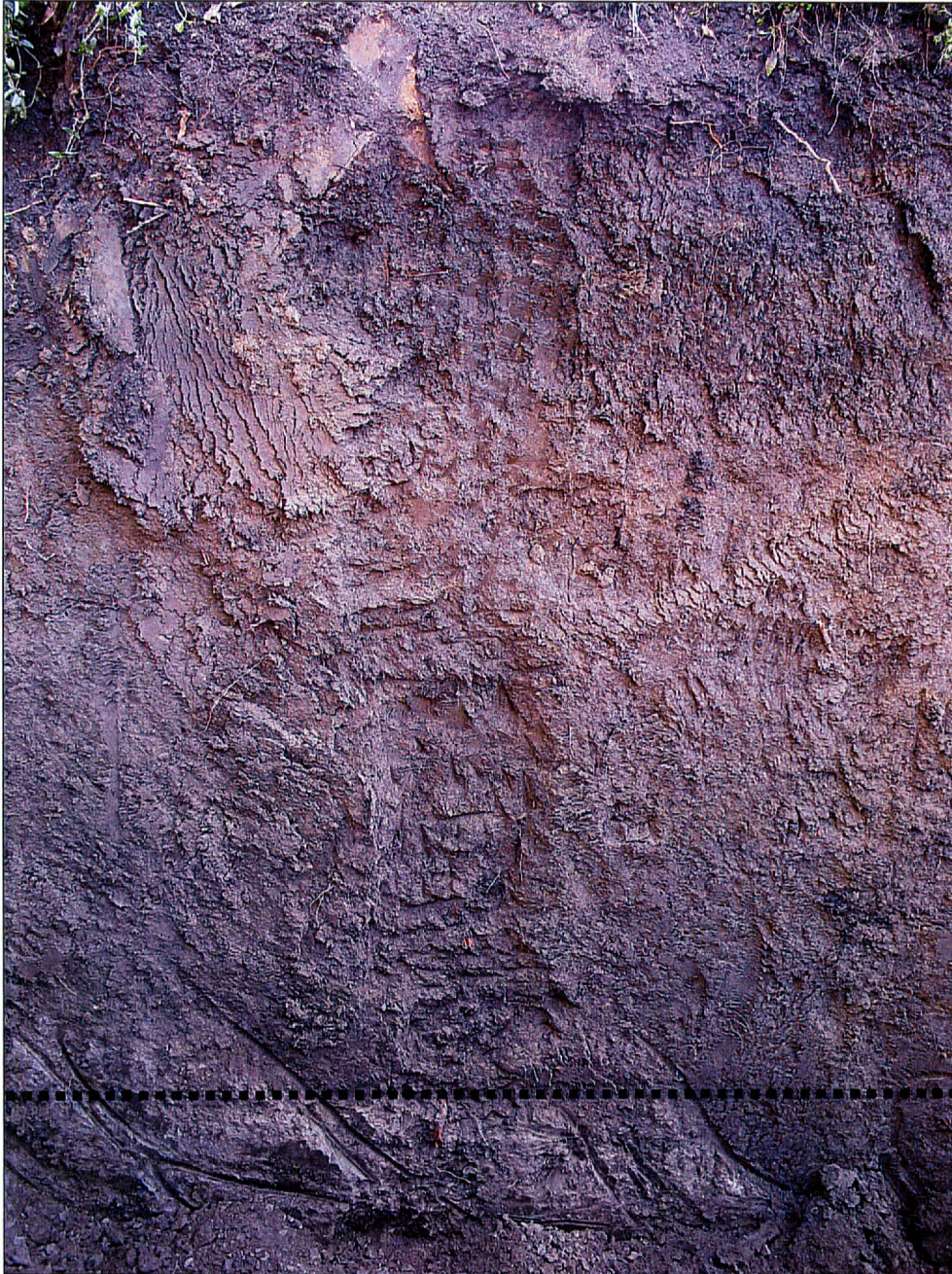
Figure 6 A Backhoe trench 3. Note the abrupt soil change in the bottom of the trench (253-310+ cm). This probably is a developing soil based on the calcium carbonate present. View is to the south.
