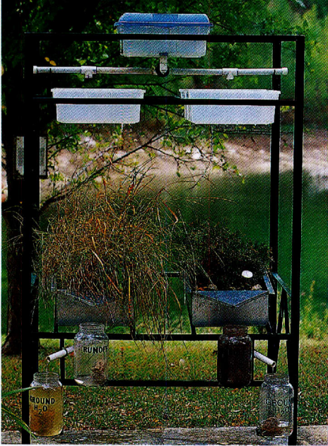
[ABOVE, LEFT] The Rainfall Machine, as it's known on the ranch, simulates the difference in rain falling on grass-covered land versus cedar scrub-covered land. Water falling on the grass slowly soaks into the "aquifers" below, with little runoff. Conversely, most rain falling on the cedar habitat runs off without recharging the aquifer.
