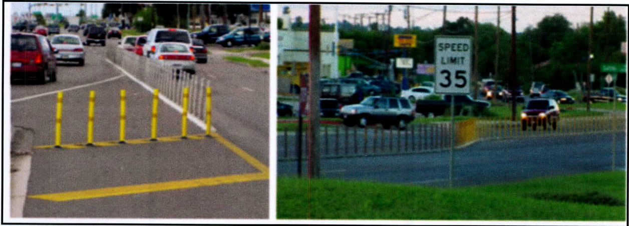
Figure 10. Access Management Applications of Pylons in Laredo, Texas: Left – Blocking Access to Driveways, Right – Delineating Left Turn Lanes.
