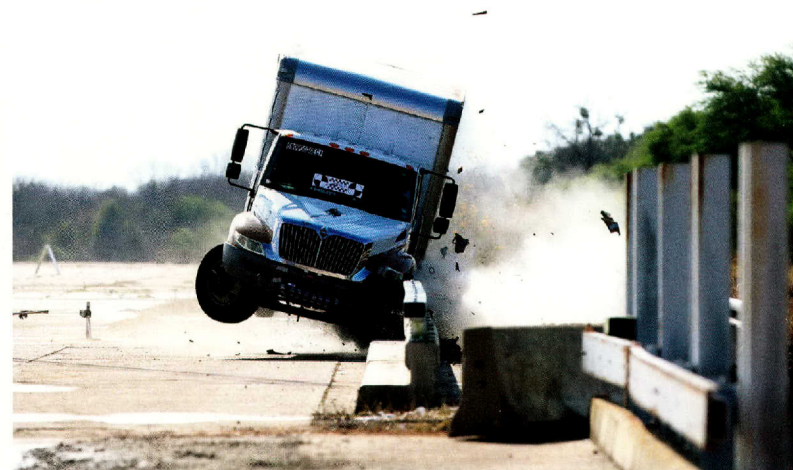
A full-scale crash test was performed at TTI Dec. 12 on one of the retrofit designs for Lake Pontchartrain.
