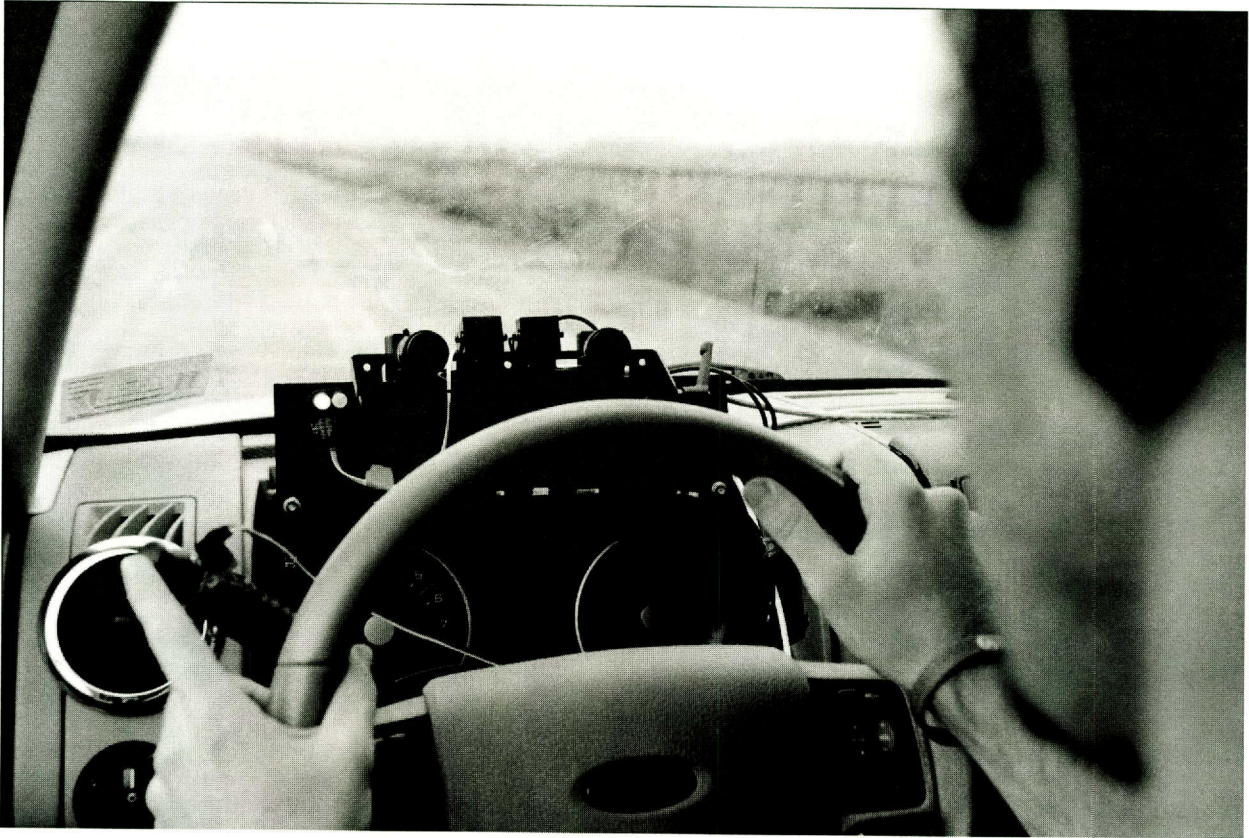
Figure 3. Dashboard-mounted light and response button
