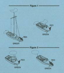
Manually Driven Vessels: Manually driven vessels when paddled, poled, oared, or windblown:
