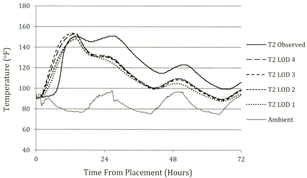
Figure 4.28: Eagle Lake—ConcreteWorks Analysis (Sensor T2)
