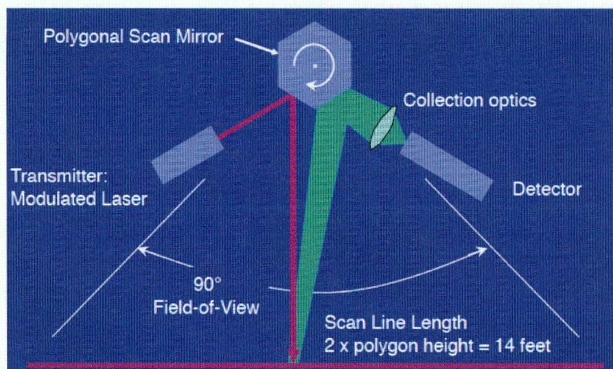
Figure 2.20: Scanning laser system scheme (Herr, 2001)
