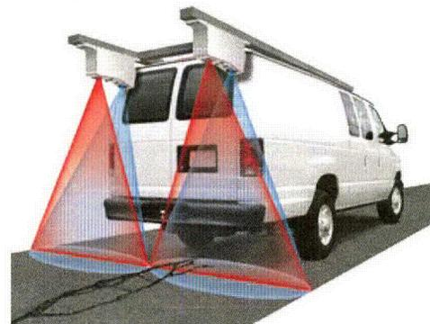
b) INO LCMS mounted on vehicle
