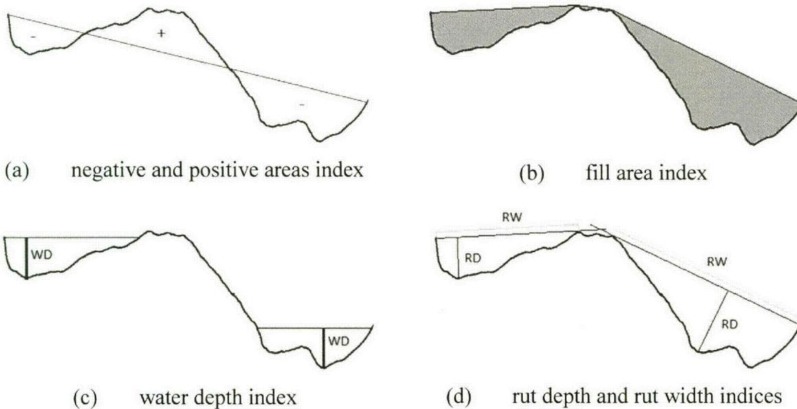
Figure 2.1: Illustration of some of the indices postulated in Simpson (2001)
