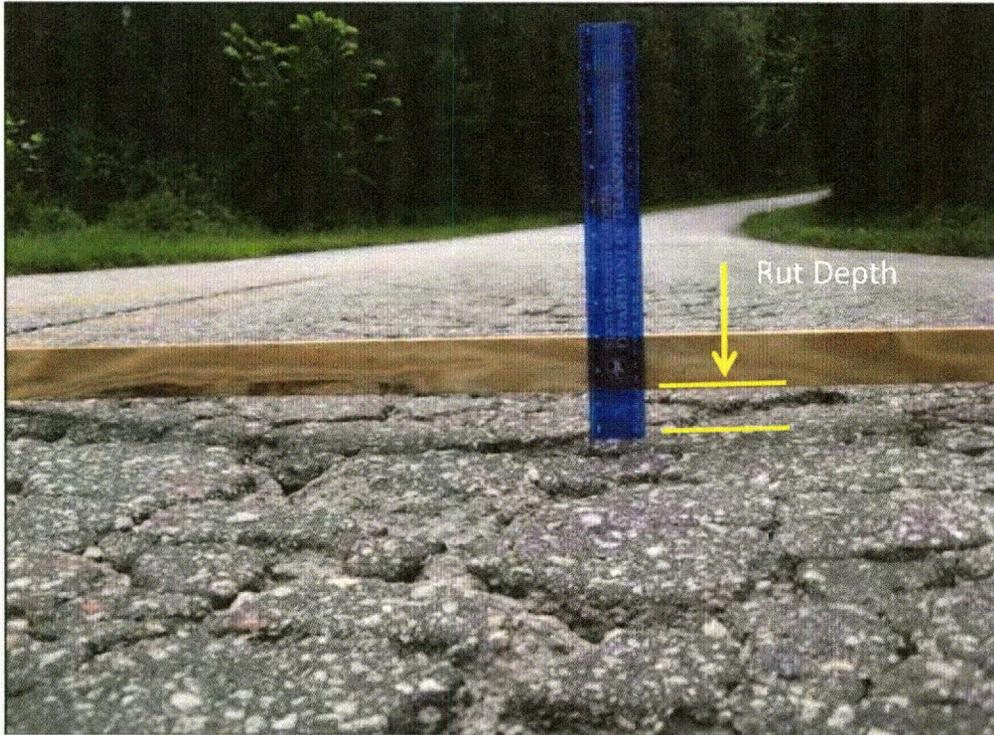
Figure 2.4: Straightedge and rut gage method field measurement
