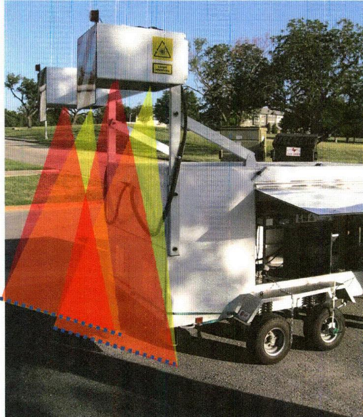
*Figure 1.7: The Applus RTD INO LCMS automated rut measurement system*
