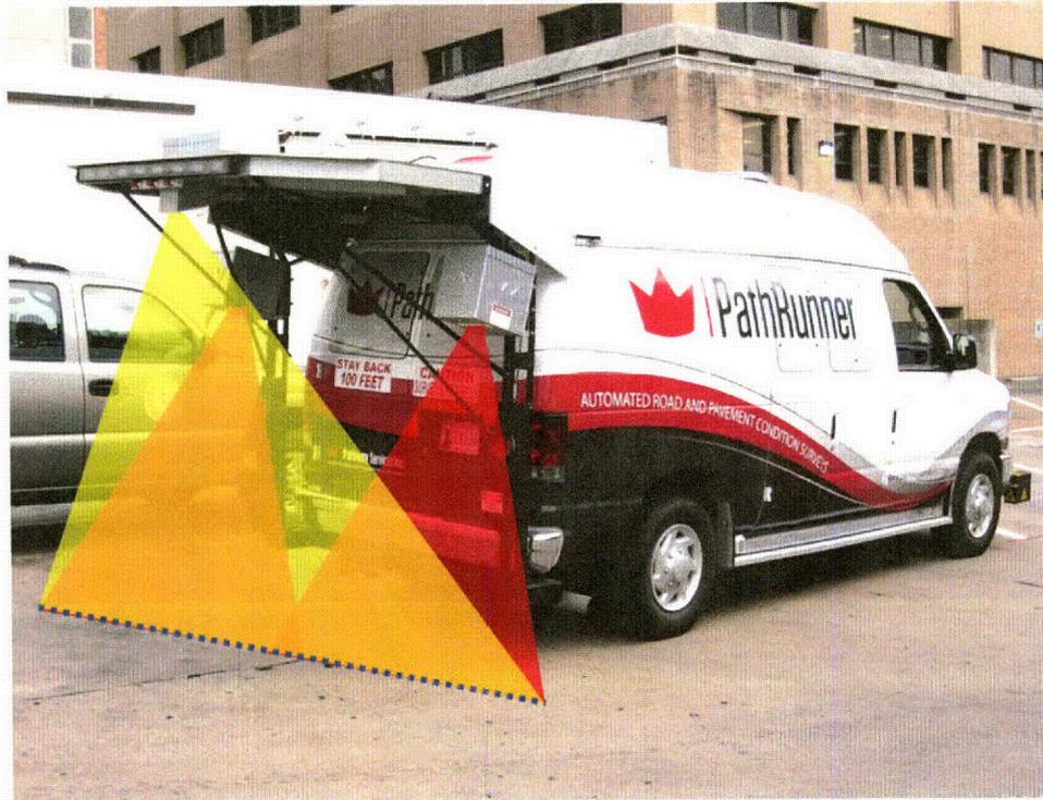
*Figure 1.4: The Pathway Services automated rut measurement system*
