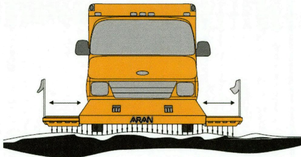
*Figure 2.6: ARAN Smart Rutbar point-based discrete system*
