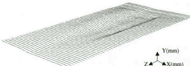
Figure 2.14: 3D Representation of the Pavement Surface (Li et al., 2009)
