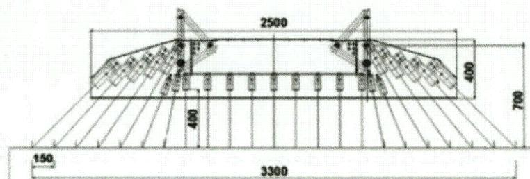
Figure 2.11: RoadSTAR fan-shaped measuring beam (Wang, 2005)
