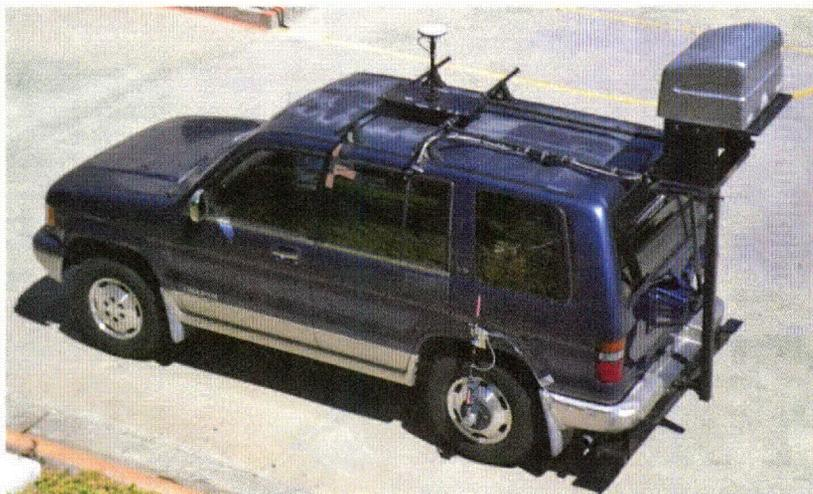
Figure 2.22: PSI PPS scanner mounted on survey vehicle (Herr, 2009)
