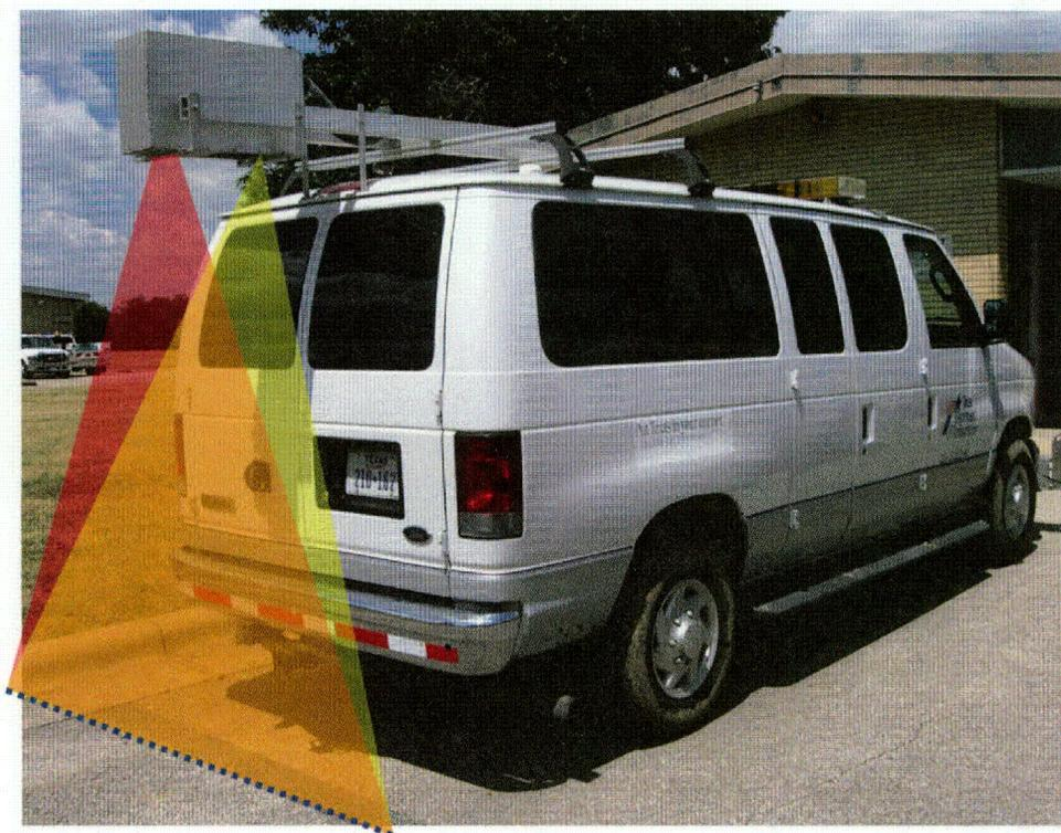
*Figure 1.3: TxDOT 3D system for automated measurement of rutting*
