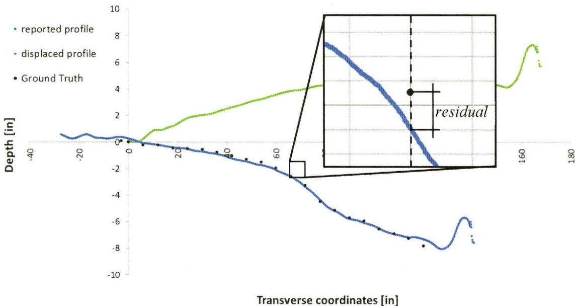
Figure 4.2: Comparison of transverse profiles
