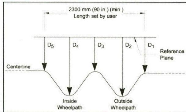
Figure 2.8: Determination of rut depths using five coordinates (AASHTO 2010)
