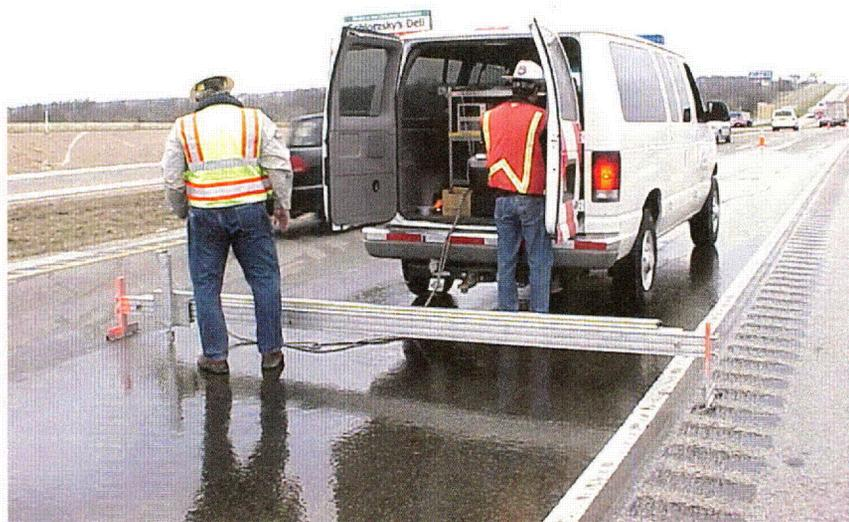
*Figure 2.2: MLS transverse profile beam used on IH 35 during an accident investigation*
