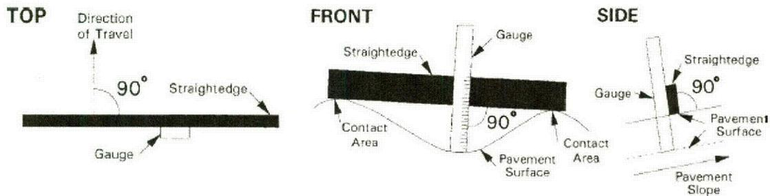
Figure 2.5: Straightedge Method (ASTM E1703)
