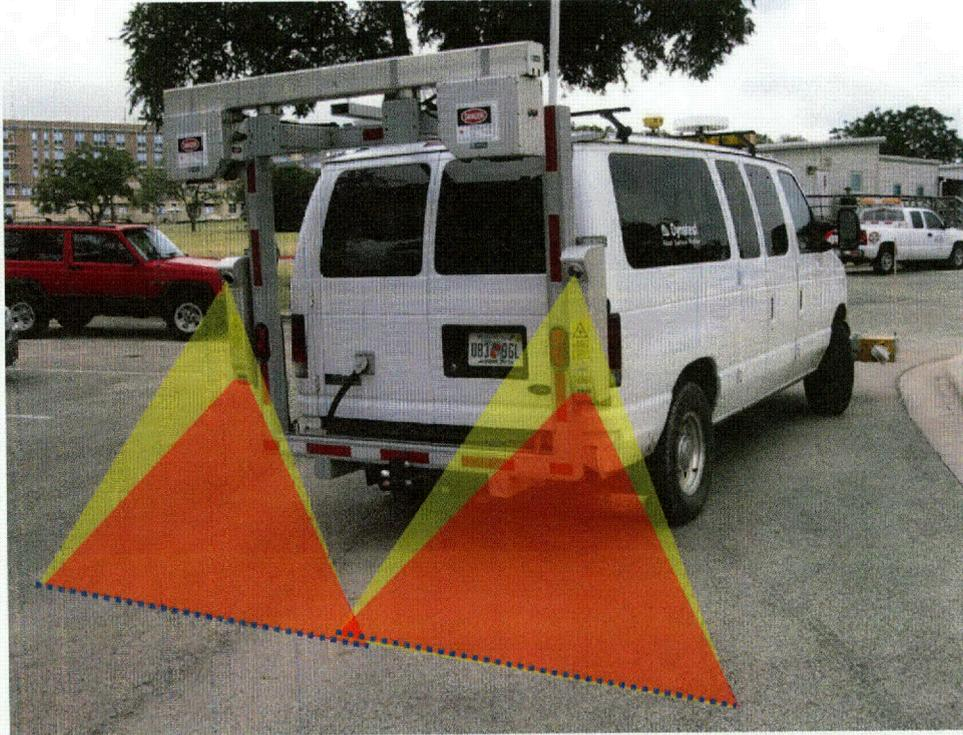
*Figure 1.5: The Dynatest INO LRMS automated rut measurement system*
