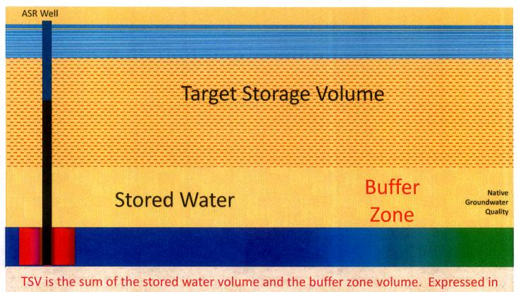
MG/MGD of recovery capacity, or in "days"
