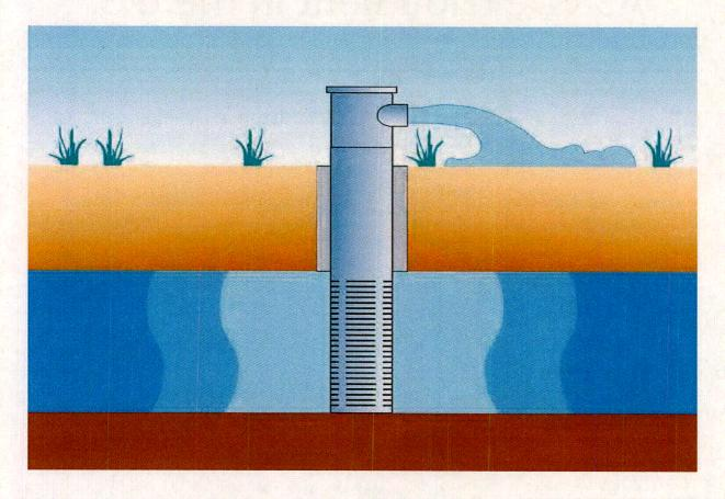
Storage of water through a well in a suitable aquifer during times when the water is available, and recovery of the stored water from the same well when needed
