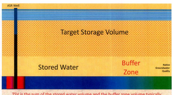
TSV is the sum of the stored water volume and the buffer zone volume, typically expressed in MG/MGD of recovery capacity, or in "days"
