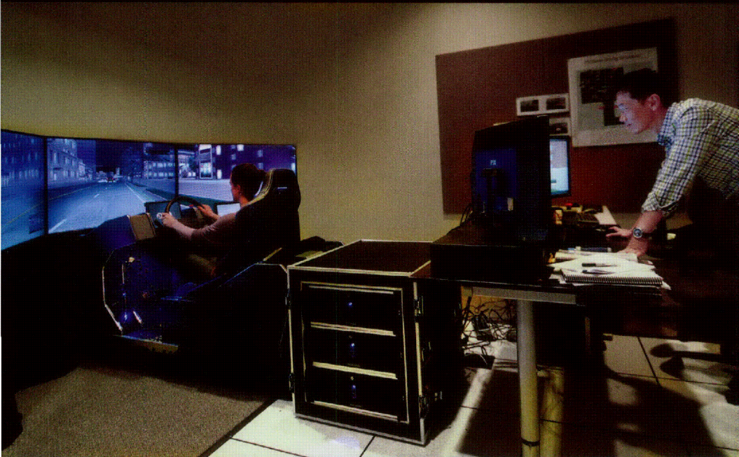
TTI researchers use a simulated driving environment to measure driver reactions behind the wheel.
