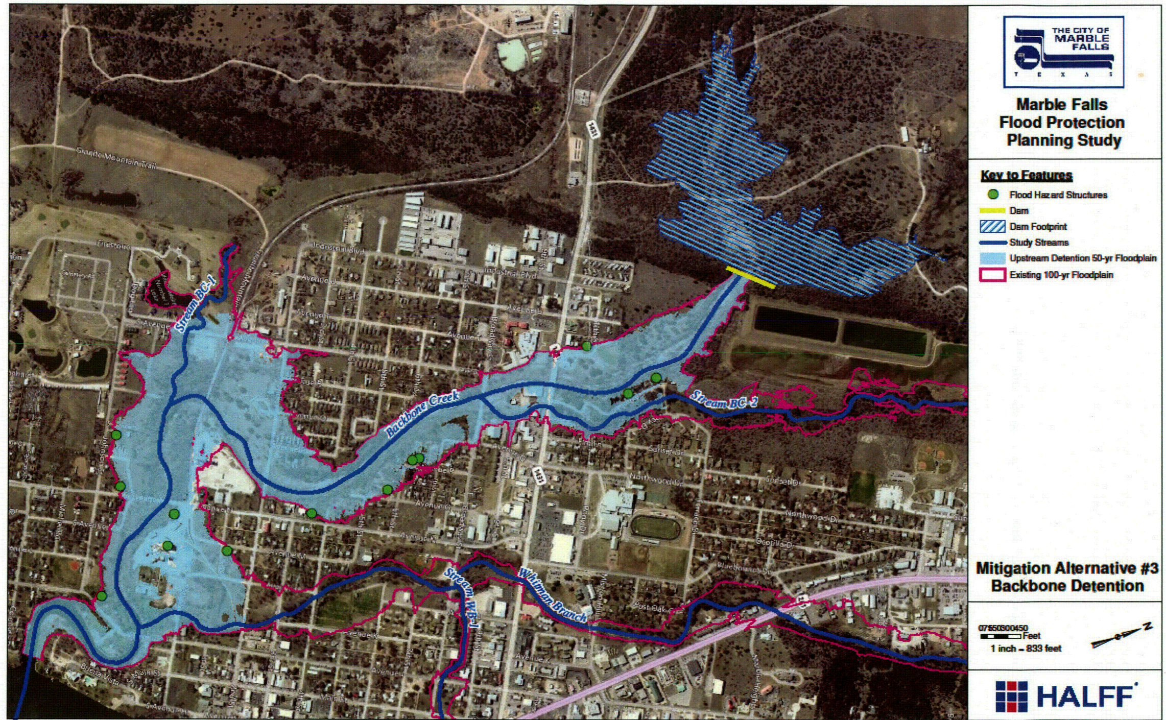
Figure B3: Backbone Detention Flood Reduction
