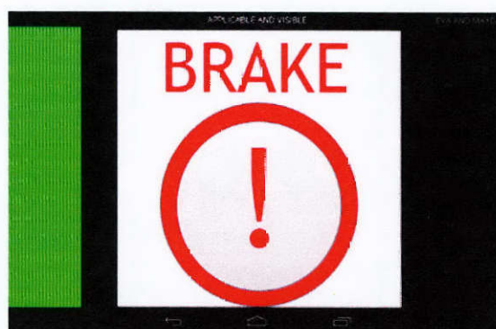
Figure 10.9: SwRI Tablet Display EEBL Message
