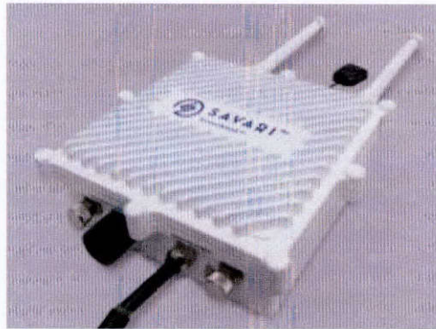
Figure 13.3: RSE DSRC Roadside Device Manufactured by Savari
