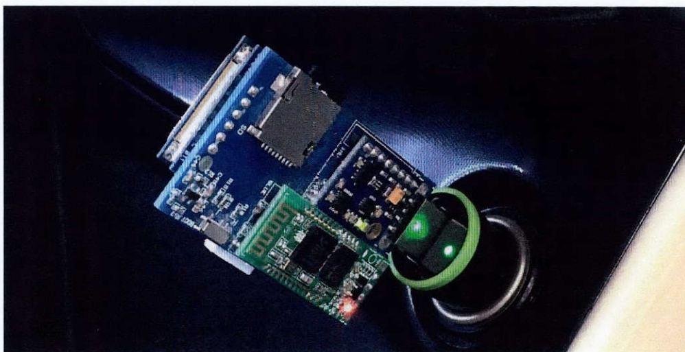
Figure 11.8: IMU Device Installed in a Vehicle, with Power Supplied through a USB Car Charger
