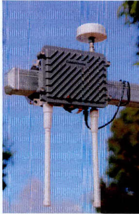
Figure 13.2: RSE DSRC Roadside Device Manufactured by Coda Wireless
