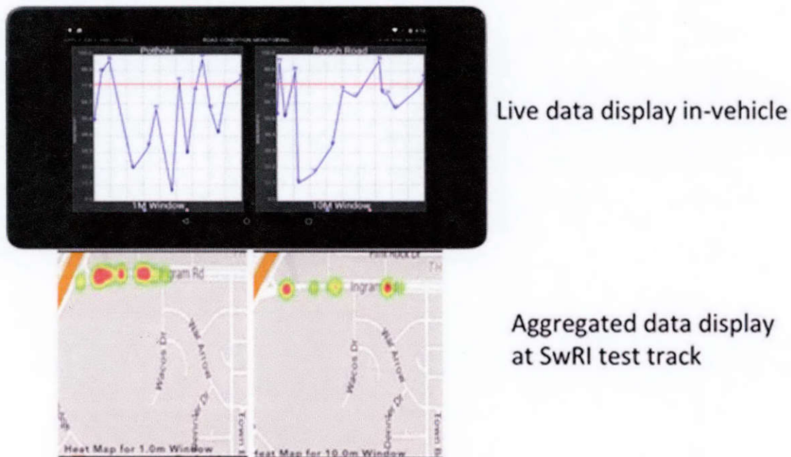
Figure 10.24: Road Condition Monitoring Tablet and Heat Map Displays
