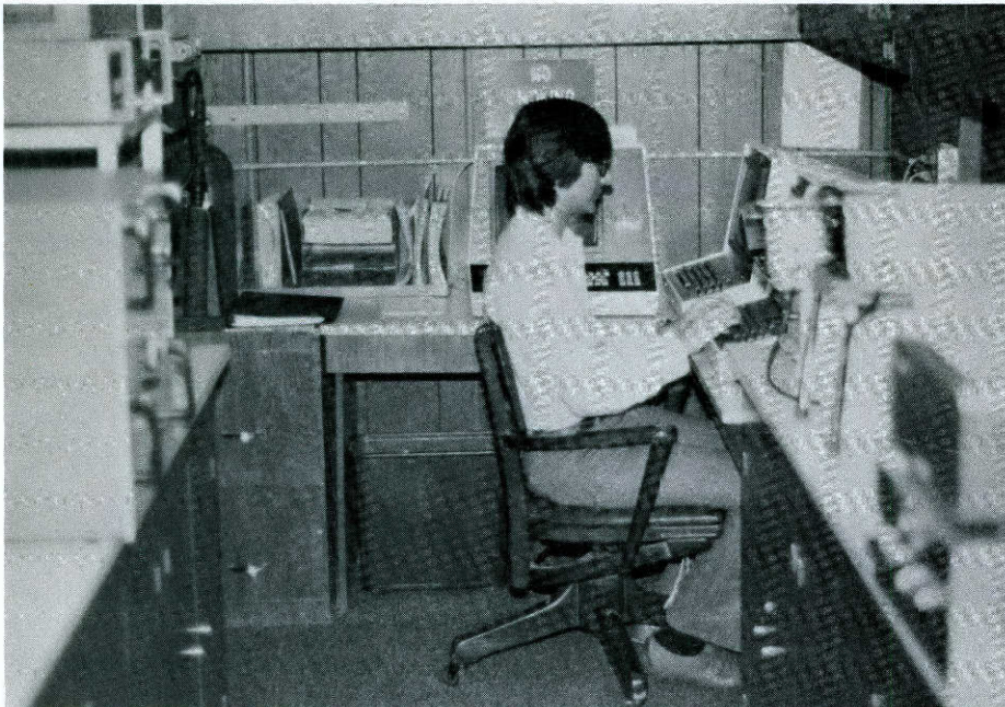
The microcomputer-based acquisition system in the automated CAMS network will provide real-time data for reporting the Pollutant Standards Index.
