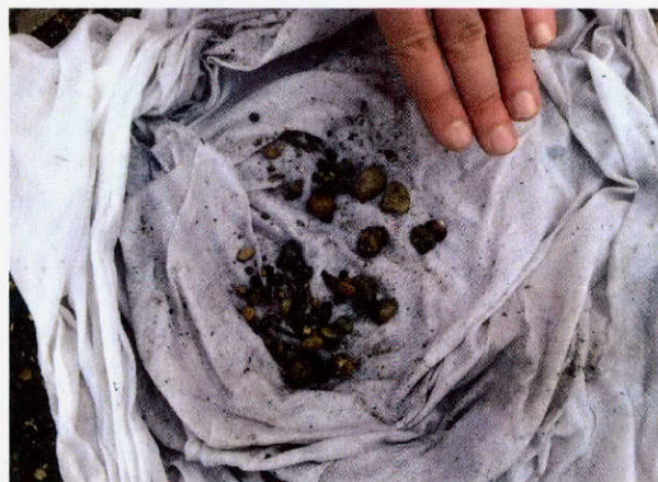
Figure 3.2: Mesh bag used for collecting HS bed sediment samples.
