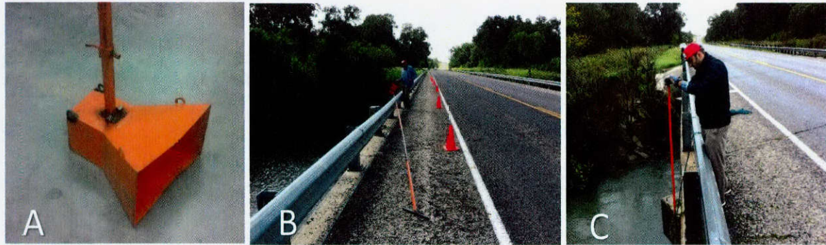
Figure 3.1: Primary sampling equipment. (A) The Helley-Smith sampler; (B) the sampler with 6 poles attached; and (C) deployment of the sampler from the bridge deck.
