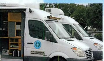
The TCEQ Air Monitoring Division has a special fleet of trucks that are essentially mobile air-monitoring stations. They are equipped with high-tech air-analysis equipment, including spectrometers and gas chromatography.
