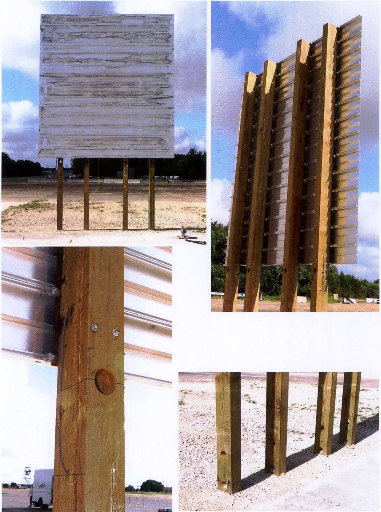
Figure 2.2. Temporary Wood Sign Support for Large Guide Signs before Testing.
