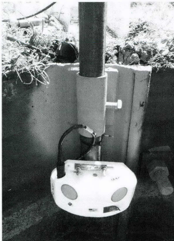
Figure 2. Sontek Argonaut SL 1500 installed at USGS streamflow gaging station 08067252 Trinity River at Wallisville, Tex
