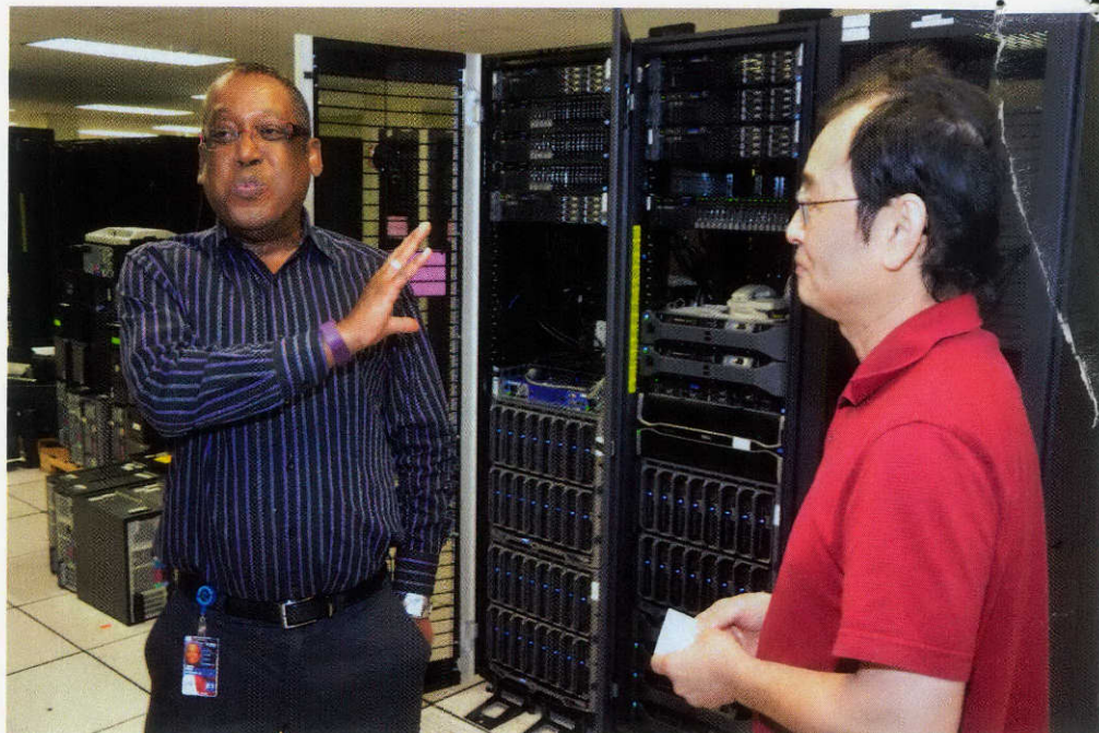
Stephen Davis, manager of the Air Modeling and Data Analysis Section, and Weining Zhao, who is the computer expert for the section, discuss the blade server that they use for air modeling. The server combines the computing power of 50 computers. "It makes it possible for us to turn around answers faster than contractors," Davis says.
