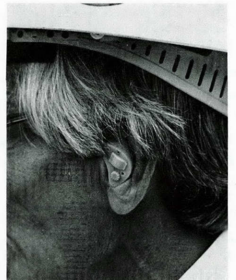
of high frequency sound. Without ear protection, more exposure to noise causes additional hearing damage. Right, Lanbright shows the custom-fit, prescription industrial amplifier that Carlin helped develop. Turning off the knob in the center makes the device into one of the best hearing protectors available. It is also more comfortable than protective earmuffs or round earplugs. When he needs to hear, Lanbright simply turns the device on for amplification of the specific tones he needs. (Photos by Gary Parker)
