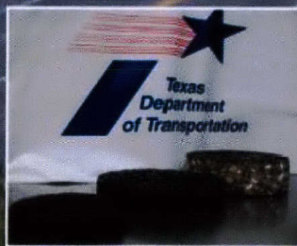
TxDOT's longer-lasting, thinner 1-inch and half-inch overlay alternatives use finer aggregates than the traditional 2-inch overlay, resulting in safer, smoother rides for motorists.
