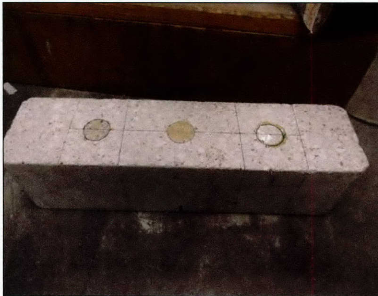
Figure 7-1: Artificial defect fabrication
