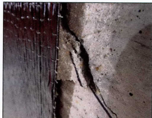
Figure 3-60: Failure of test 48-3-14-8
