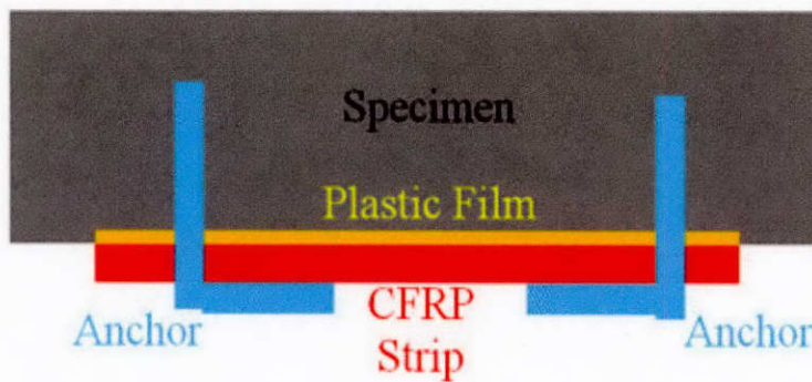
Figure 6-19: Layout of unbonded specimens
