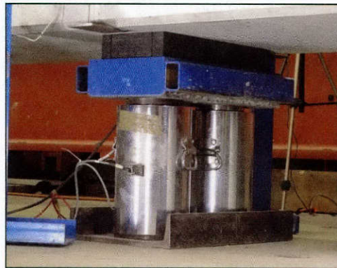
Figure 5-10: Reaction in the test region (2-1000 kip load cells)
