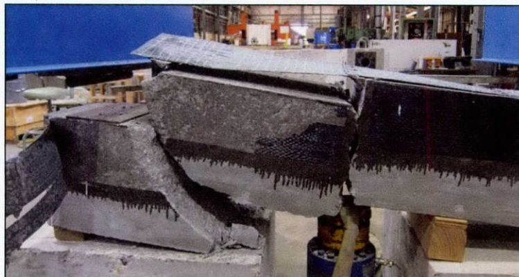
Figure 6-26: Beam specimen failure
