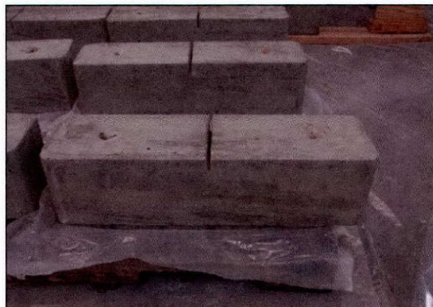
Figure 6-2: Beam specimen before CFRP installation (Series 1 to 3)
