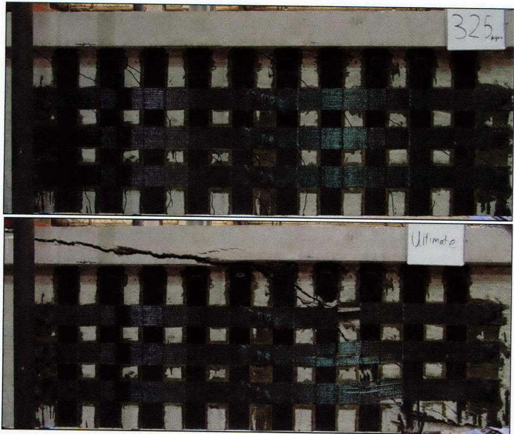
Figure 3-63: Test 48-3-14-9 before failure (top) and after failure (bottom)
