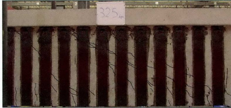
Figure 3-48: Cracking pattern of 48-3-14-3
