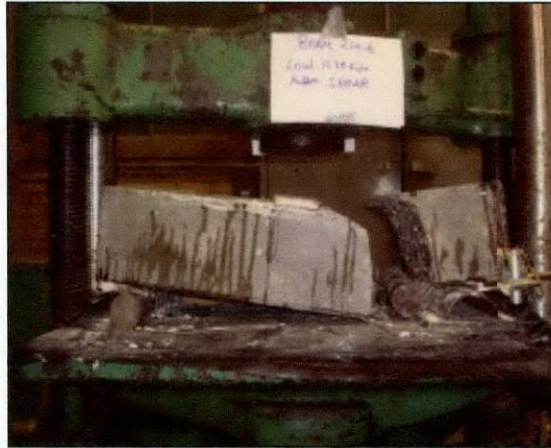
Figure 5-17: Concrete beam shear failure (Huacc, 2009)
