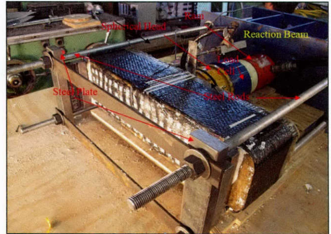
Figure 6-38: Loading and test setup for series 1-3
