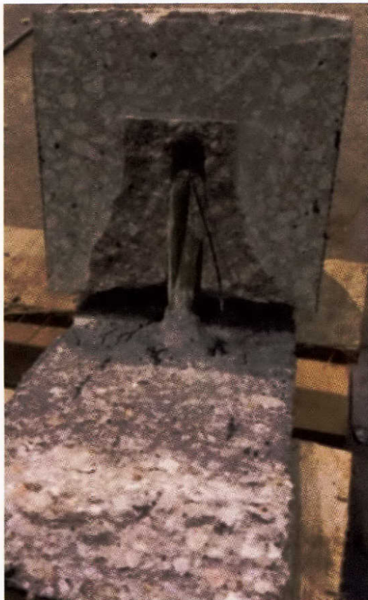
Figure 6-54: GFRP pullout, sectional view
