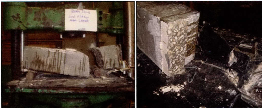
Figure 6-41: Concrete beam shear failure (Huaco, 2010)
