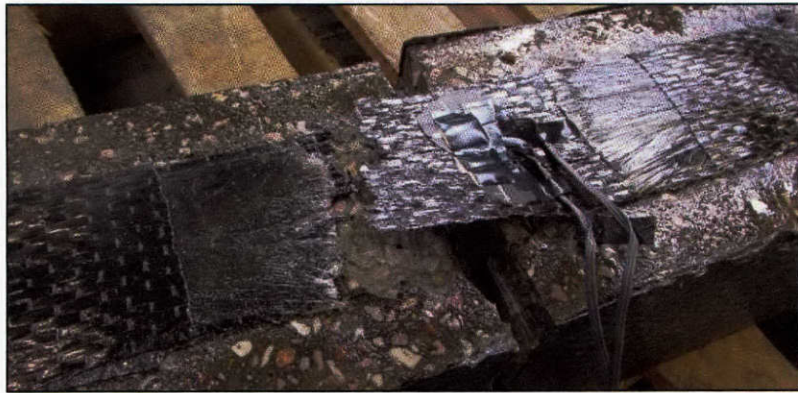
Figure 6-53: CFRP strip fracture
