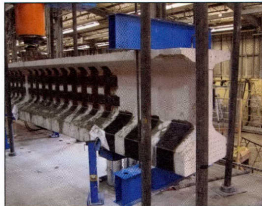
Figure 4-9: Strengthening of the cut end
